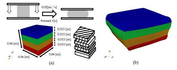
Figure 1: Problem pressing the laminate stacked vertically; (a) Simulation condition and (b) Result.
