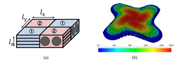
Figure 2: Problem pressing the laminate placed on a checkered pattern; (a) Simulation condition and (b) Result.
